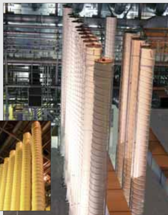
Below and Inset: American Centrifuge machines operating in a cascade configuration at the American Centrifuge Demonstration Facility in Piketon.
