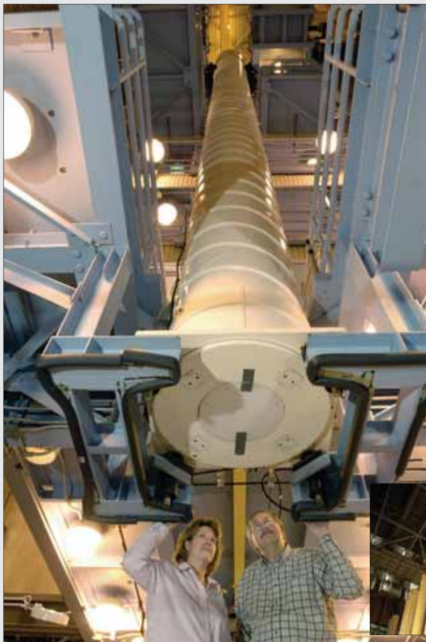
Below and Inset: American Centrifuge machines operating in a cascade configuration at the American Centrifuge Demonstration Facility in Piketon.
